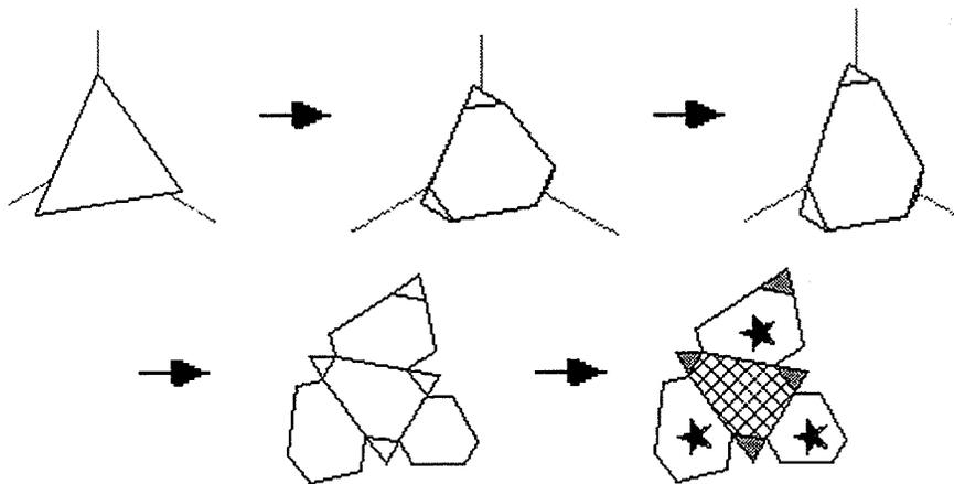
**Figure 1:** (*Top row*) A tetrahedron is truncated, then stretched. (*Bottom row*) A folding net is produced for the new shape; this net is then decorated with solid colors, patterns, and turtle graphics. The decorated shape may now be printed and folded into the desired solid.
