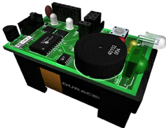
Figure 8. A diagram of the cricket. The two actuator output ports and sensor input ports are at the far side of the surface, toward the left. The infrared output and input are positioned along the right edge of the cricket. A standard 9V battery as power supply is housed underneath the device (which should also give the reader a sense of the object's scale).
